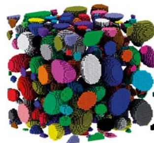
Microscopic representative volume cell of a casting slurry (only solid particles are illustrated).
