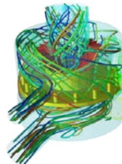
1 *Multiphase flow inside an air classifier mill.*
