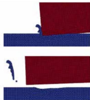
1 Simulation of a solid grain (red color), which impacts an aluminum workpiece (blue color). In this case, the workpiece is plastically deformed and a chip is separated due to ductile material failure.
