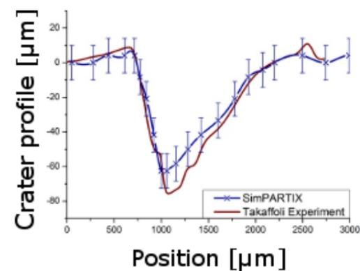
2 The comparison of simulation and experiment (Takaffoli et al., *Wear*, 274–275:50–59, 2012) underlines the quality of the numerical modeling.
